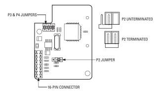
Figure 2. TXB-V Termination and Baud Rate (Bottom View)
